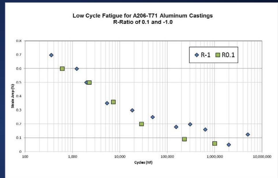
Material Source: Test specimens machined from chilled sand cast test plates
